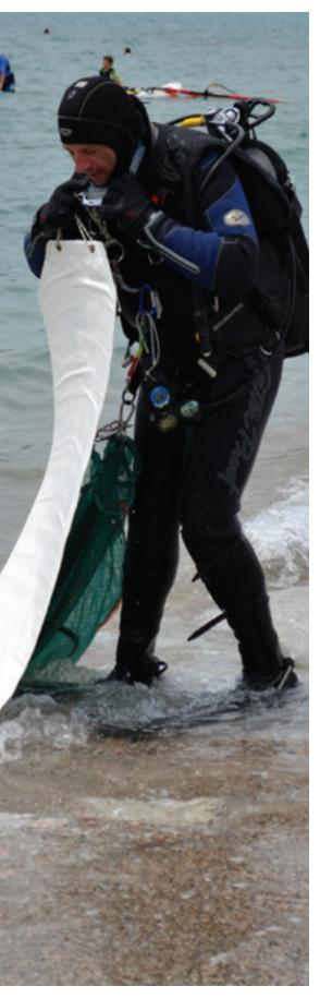
out a 100-metre tape measure or alternatively by laying a 100-metre rope across the bottom. The start and end point of each transect were identified with marker buoys and recorded using a GPS.
