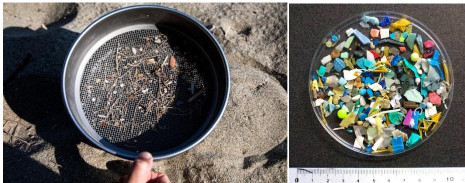
Figure 13: Material retained on the 5 mm sieve (left), plastic items larger than 5 mm (right).
