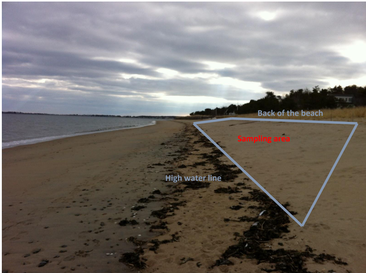
Figure 9: Blue square indicates appropriate location for beach sediment microplastic sampling (between high water mark and back of the beach)
