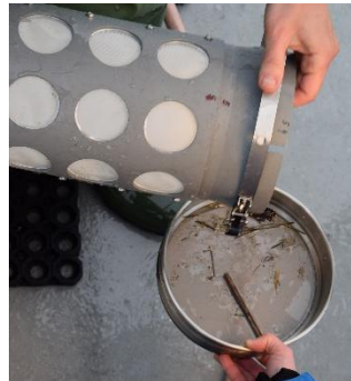
Figure 4: Sieving the sample from the cod end (photo: IWRS).
