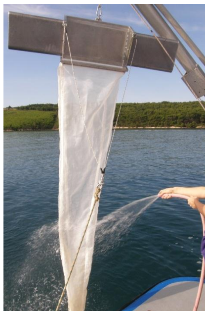
Figure 3: The manta net rinsing (photo: IWRS).
