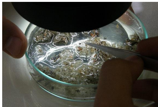
Figure 6: Sample analysis by the stereomicroscope and tweezers (photo: IWRS).
