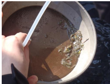
Figure 5: Concentration of the material in one part of the sieve (photo: IWRS).
