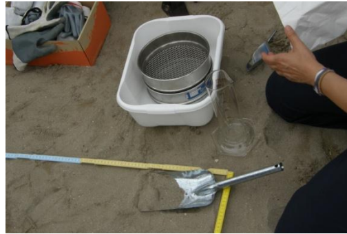
Figure 12: Collecting the top 3 cm of sand with a metal scoop.
